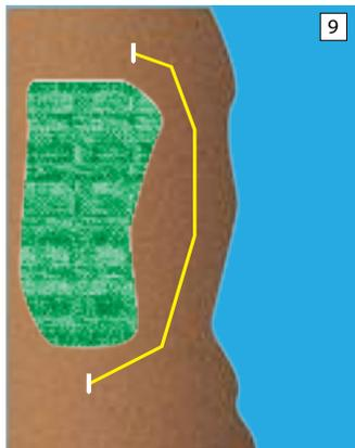
A staked barrier is designed specifically for locations dealing with high water flow. It is primarily used to control and direct storm water or sheet flow to sediment settling ponds or retention basins. Staked silt barriers function best in porous soils on sloping grades as shown in Figure 9.
