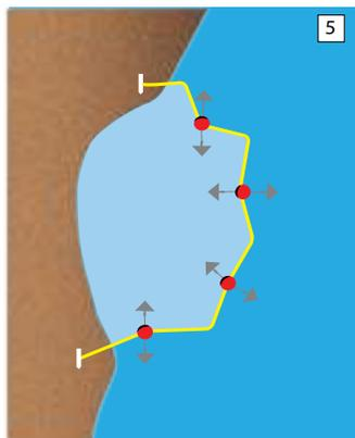
In areas with flowing water, dual anchoring is recommended so that the orientation of the silt curtain remains parallel to the flow. Figure 5 displays a barrier system in a tidal environment. When anchoring the curtain in tidal or other conditions that may be subject to loading from either side, it is best to anchor from both sides so that a wind or current change doesn't override the effectiveness of the anchors.
