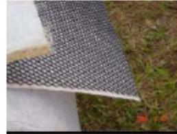
Geocomposite for drainage
