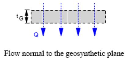
Geotextile filters have to attend criteria that assure that the base soil will be retained with unimpeded water flow. Available retention criteria establishes that
