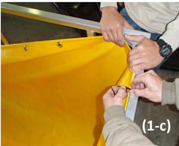
**Step 5:** Lace the rope through the grommets and around the frame. (1-d)
