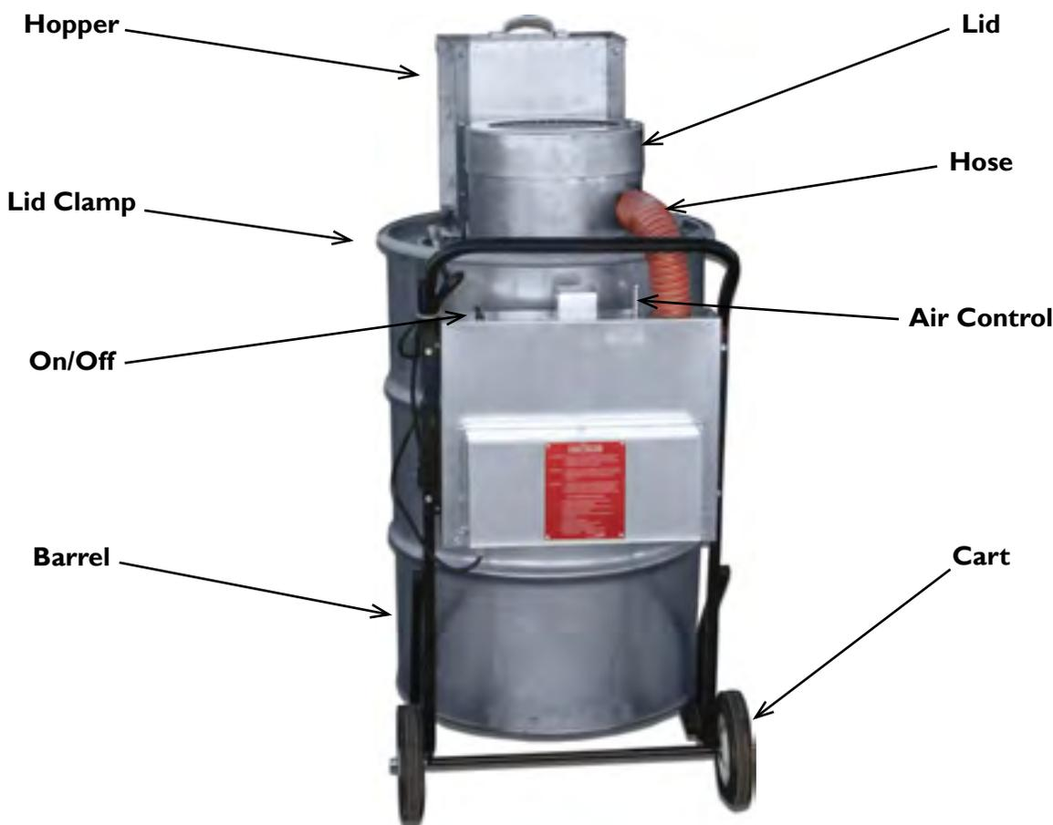
**Assembled unit includes the stainless steel drum, cart, blower, lid, controls, hopper and air hose.**
